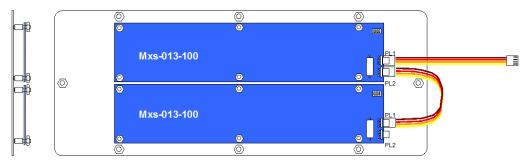
The Mxp-013-200 consists of 2x 100 LED Indicator cards mounted on the fascia plate and connected together using an interconnecting ribbon cable.
