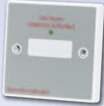
A low-cost remote indicator incorporating a red LED. Ideal for indicating the activation of out-of-sight smoke or heat detectors (in lift shafts, hotel bedrooms, etc.) or fire alarm sounder circuits. Three inputs are provided 'OV', '+30V d.c.' and 'LED only'.
