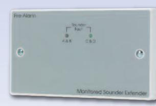
Compatible with most fire alarm panels, the FF502P can be connected to any unpopulated sounder circuit to provide four extra sounder circuits with open and short circuit monitoring, two trigger inputs and one fault output. The four
