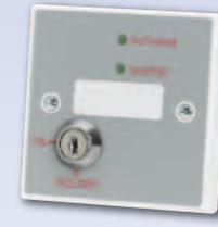
Combines the functions of the BF376 general purpose 5A relay (above) and the BF367 keyswitch operated device isolator (left) in a single unit. Includes a double-pole relay capable of switching loads of up to 240V a.c at 5A and a keyswitch isolation facility that allows the relay operation to be temporarily disabled during routine test and maintenance. Mounts on 25mm UK single gang back boxes.
