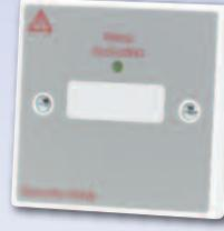
A cost-effective double-pole, polarised changeover relay that is capable of switching loads of up to 240V a.c at 5A. Incorporating a red LED which illuminates when the relay is active, the BF376 may be connected to a suitable control panel relay output or a standard polarised sounder circuit to operate door retaining magnets, rollershutter doors, etc\*. Mounts on 25mm UK single gang back boxes.
