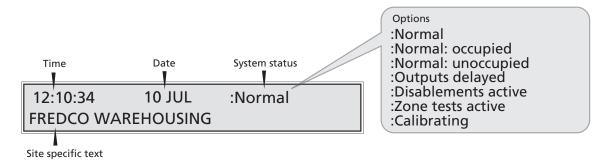
**Normal** is displayed when there are no fires, faults or pre-alarms on the system and the panel's day/night (building occupied/unoccupied) facility HAS NOT been set up by the system engineer.
