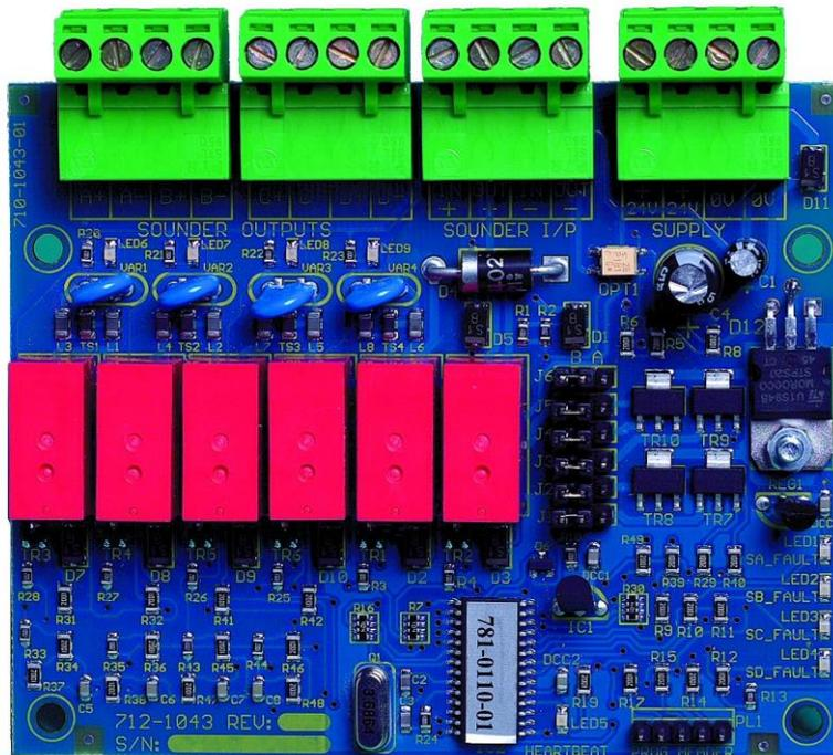
The Mxp-021 Sounder Circuit Splitter is a peripheral unit for use with all of the MxPro 4 range of control Panels.
