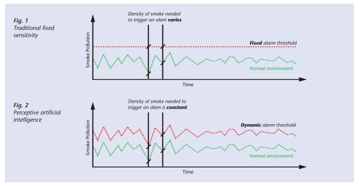
ClassiFire® dynamically adjusts the detector sensitivity to match changes in the normal environmental smoke density, thus the amount of smoke needed to generate an alarm remains constant, irrespective of environmental conditions.
